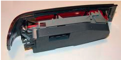
Tail-lamp assembly. The lens and bulb carrier both attach to the reflector.
